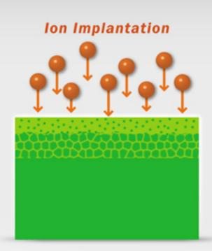
The ion implantation step damages silicon crystal structure, causing it to become amorphous.
