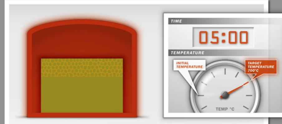
At the target temperature, the amorphous silicon layer crystallizes into the desired polycrystalline layer.
