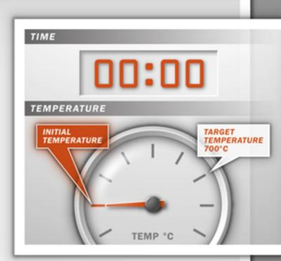
Substrate with amorphous silicon layer is held at initial temperature to achieve a thermal equilibrium.
