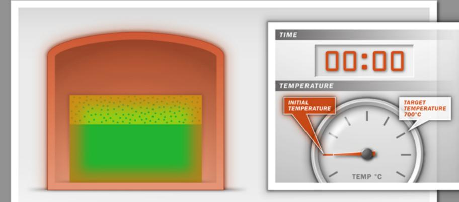
Substrate with amorphous layer is heated to an initial temperature that is LOWER than the crystallization temperature.
