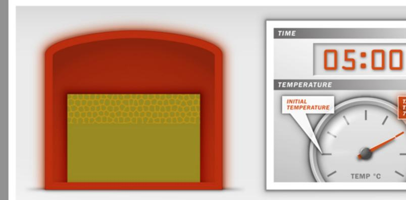
The controlled heating causes recrystallization into a polycrystalline layer having a defined grain size and texture.
